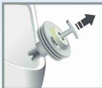
STEP 1 Remove old valve with service key
