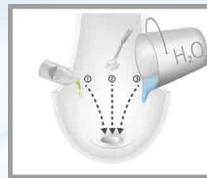
STEP 2 Flush with a 10 ltr bucket of water containing recommended Bacterial cleaner & fizzy drain tablet
