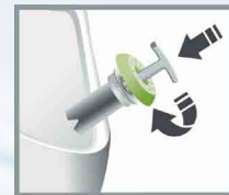
STEP 4 Insert new Key Valve and activate with 1 litre of clean water as per instructions.
